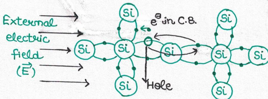
At very low temp., the valence  $e^-$ 's are stably located in the bonds of a Si crystal. However, as temp  $\uparrow$  due to thermal excitation, some of the  $e^-$ 's may get dislodged from a bond and get into the conduction band, leaving a vacancy in the V.B. (hole)
